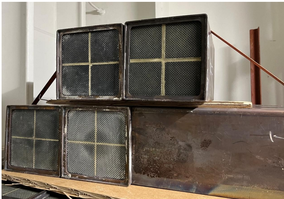
Figure 1.1: A used wall-flow diesel particulate filter (DPF) filter elements taken out of the filter housing onboard a marine vessel.
