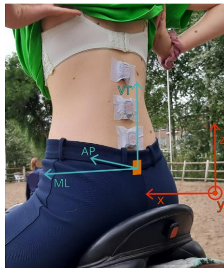
Figure 1. IMU placement and schematic representation of the local IMU frame (in blue) and the global frame (as in ISO 2631-1:1997 [10], in red). The pelvis IMU is drawn in, as it is covered by the pants.
