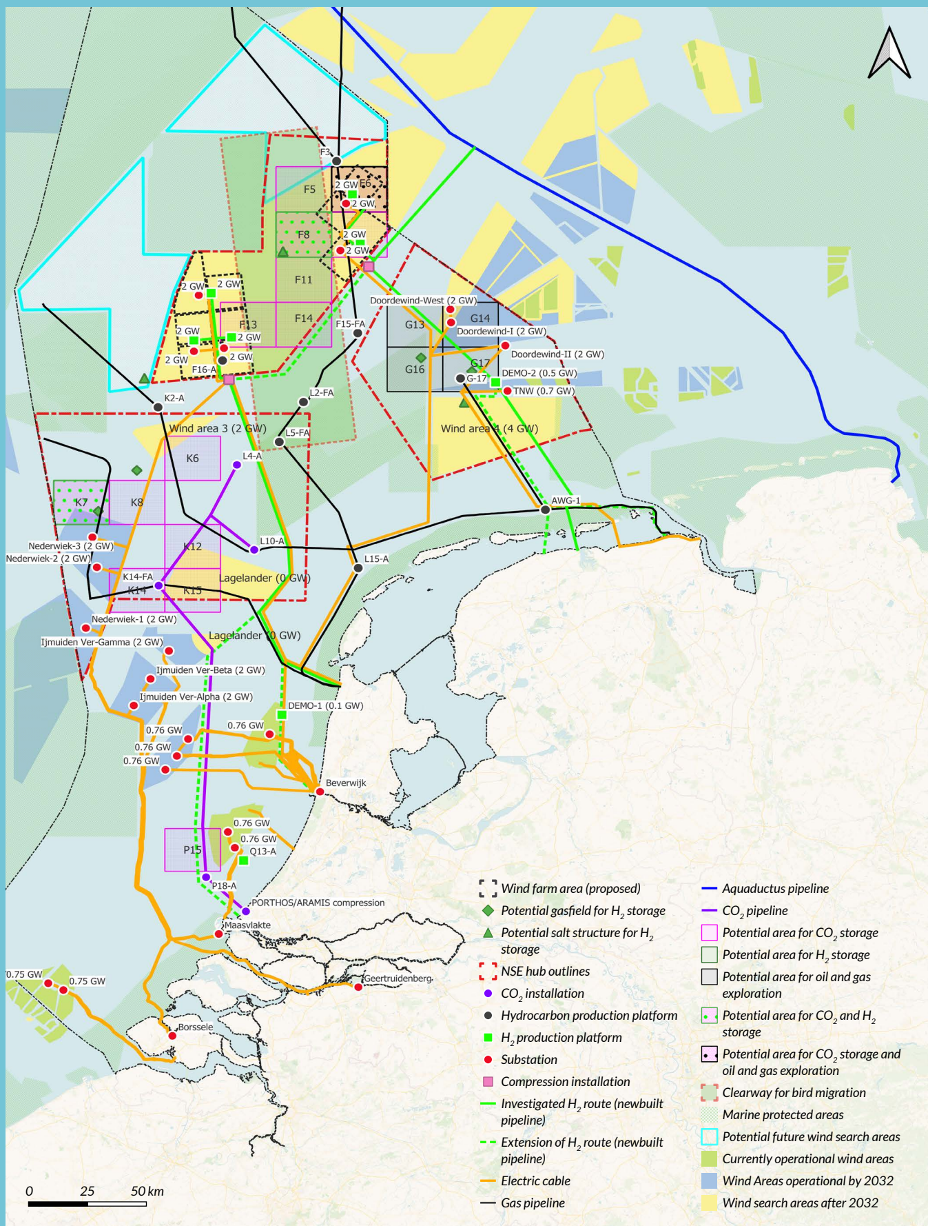
Figure 2: Vision of the North Sea in 2050 with blueprints of the three NSE hubs according to the ambitious NSE5-NAT scenario with 70 GW offshore wind and 20 GW offshore hydrogen production, and transport infrastructure of electricity and hydrogen (all new built in this particular scenario).
