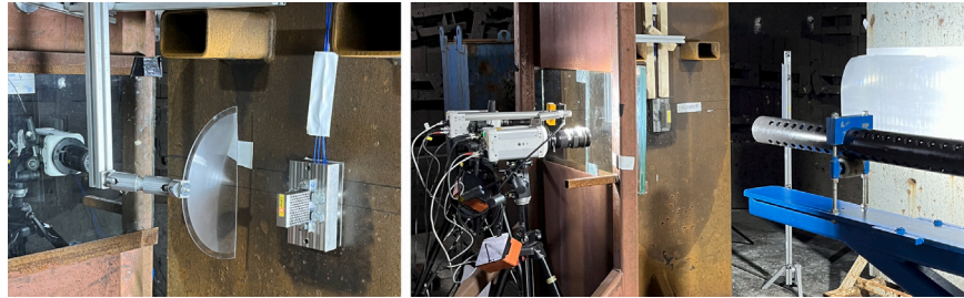
(a) Position of the camera with Fresnel (b) Shooting barrel and camera pointing at the sample. lens.
