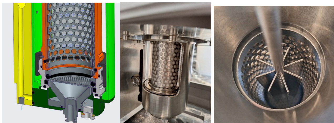
Figure 4: Foam rheology measurement cell with perforated wall and drainage opening and measurement spindle.
