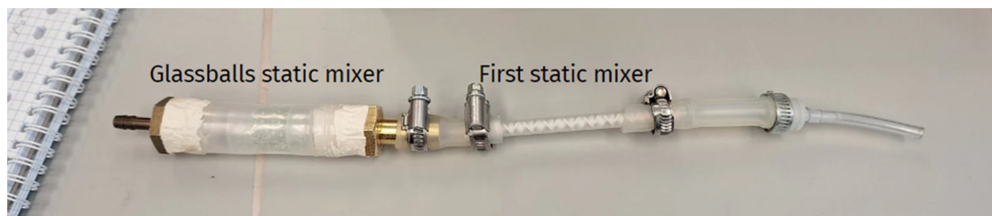
Figure 3: Home-build static mixer for foam generation.
