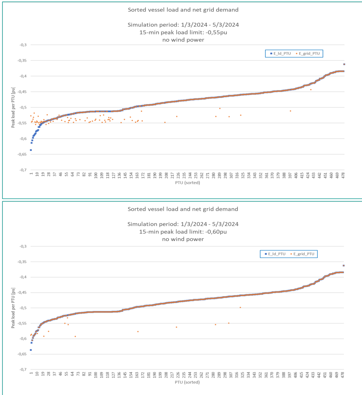
Figure 4.5: Sorted vessel load per PTU (blue) with resulting grid demand (orange) for two simulation cases (peak load limit -0.55pu and -0.60pu)
