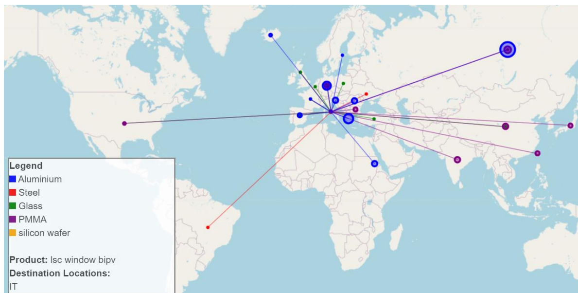
Figure 61 Visualization of the location of the major suppliers of the main materials required to produce 1 square meter of LSC window BIPV product. The dimension of the circle is directly proportional to the GHG emissions required from electricity to produce the amount of material required
