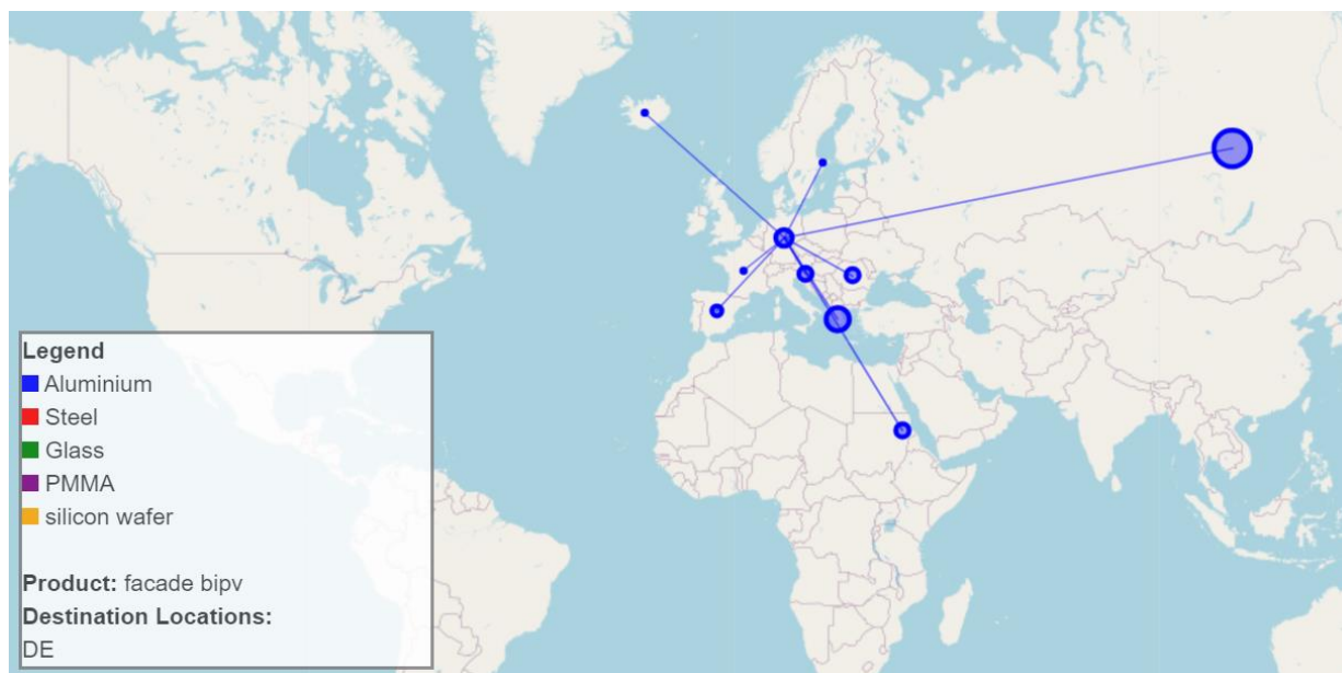
Figure 62 Visualization of the location of the major suppliers of the main materials required to produce 1 square meter of façade BIPV product. The dimension of the circle is directly proportional to the GHG emissions required from electricity to produce the amount of material required
