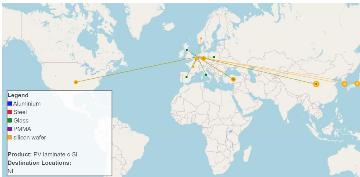
Figure 58 Visualization of the location of the major suppliers of the main materials required to produce 1 square meter of c-Si PV laminate. The dimension of the circle is directly proportional to the GHG emissions required from electricity to produce the amount of material required
