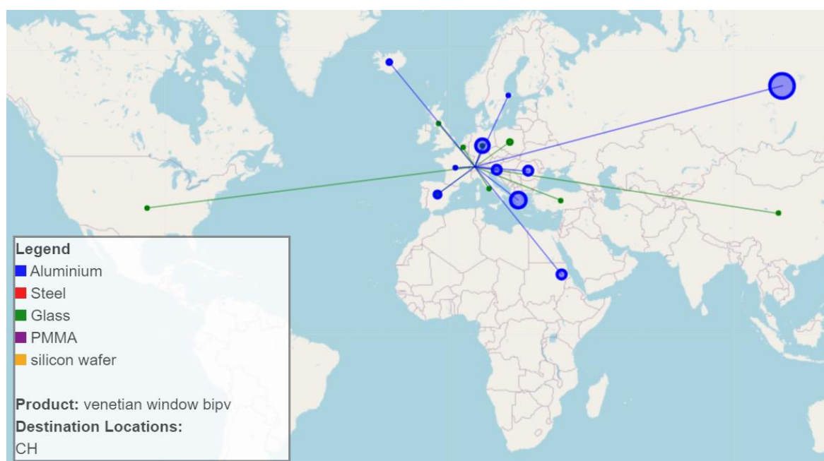
Figure 59 Visualization of the location of the major suppliers of the main materials required to produce 1 square meter of venetian window BIPV product. The dimension of the circle is directly proportional to the GHG emissions required from electricity to produce the amount of material required
