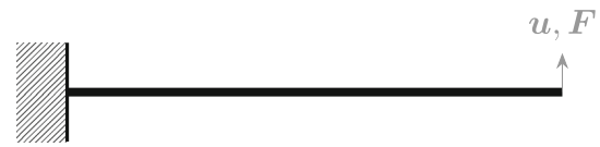
Fig. 2 Schematic of a cantilever beam under load
