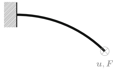
Fig. 8 Schematic of a bent cantilever beam under load
