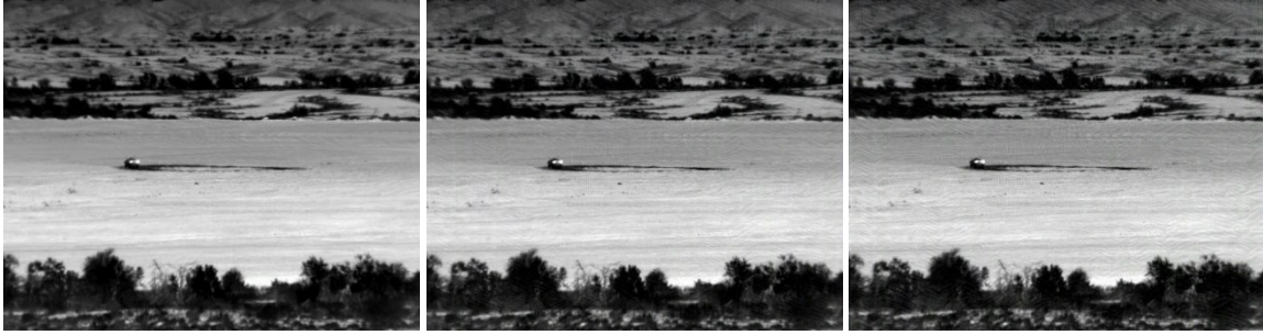
Figure 3. An example of a BRM-2 on the MWIR daytime imaging at a distance of 1500 m. Left: the original image is without any adversarial perturbation patch applied. Middle: patch with L_\infty norm of \frac{8}{255} applied, which is visually not very noticeable. Right: patch with L_\infty norm of \frac{11}{255} applied, which is somewhat noticeable visually. The raw patch itself is provided in Figure 1. Images are best viewed on a computer screen after zooming in.
