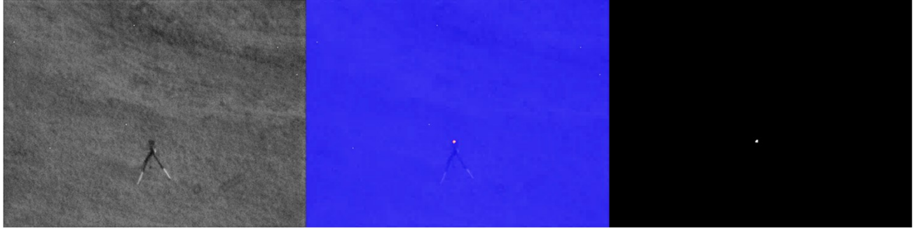
Figure 10: The laser retro-reflection captured by an event camera, from left to right, the background, the event rate heatmap overlapped with the background image, and the detection mask
