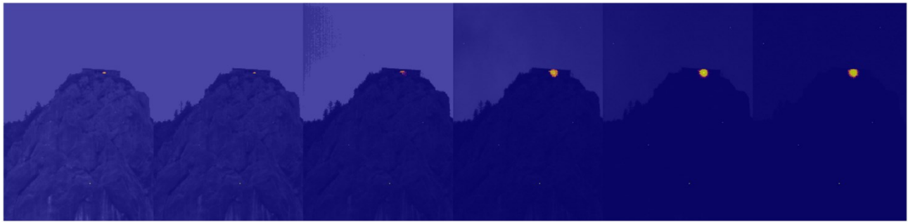
Figure 5: The event rate heatmap for different aperture sizes. From left to right, f/2.8 , f/4.0 , f/5.6 , f/8.0 , f/11.0 and f/16.0 .
