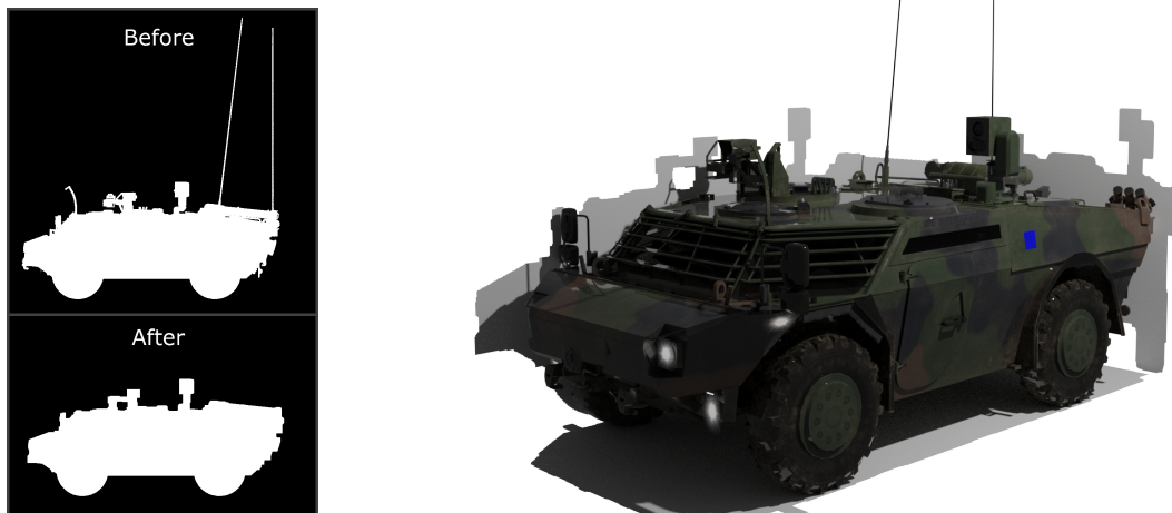
Figure 2: Left: The silhouette over the X-axis of the 3D model before and after the opening operation. Right: The complete model with refined silhouettes, vertices outside the silhouette boundaries will be removed.
