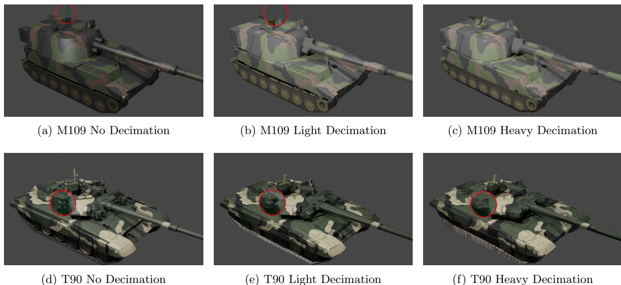
Figure 3: Comparative visualization of M109 and T90 models under different decimation settings. The top row shows the M109 model from no decimation to light and heavy decimation settings, while the bottom row shows the T90 model with similar variations. The red circles in the top row show that antennas are removed in the decimation step of the M109. In the bottom row, the smoke grenade launchers of the T90 are highlighted, which are gradually simplified in the decimation steps until only a cube with a textured surface remains.
