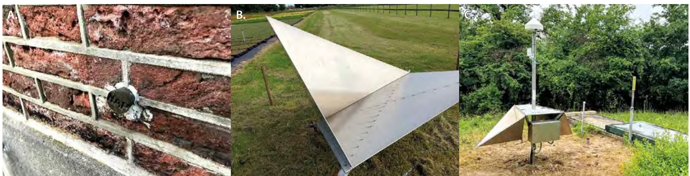
Figure 23.8. Physical benchmarks. a) the Amsterdam Ordnance Datum NAP ('Normaal Amsterdams Peil') at Noordeinde, Delft. b) A corner reflector for InSAR satellite data. c) Integrated geodetic reference station (IGRS) with GNSS antenna on the mast, airborne laser scanning horizontal platform, levelling benchmark, and two corner reflectors.
