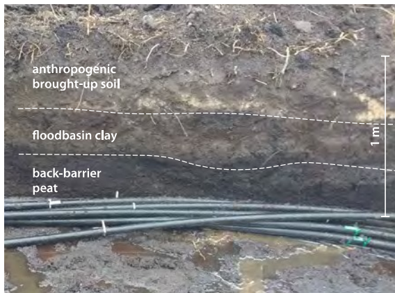
Figure 23.5. Example of anthropogenic brought-up soil in the urbanized area of Amsterdam (from Koster et al., 2018). The overburden of the brought-up soil causes underlying peaty and clayey substrate to compact and leads to subsidence.
