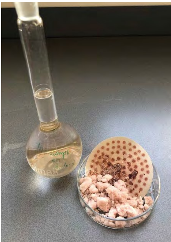
Figure 19.19. Example of the amount of salt precipitated from 100 ml of geothermal brine from the Koekoekspolder geothermal system after evaporating the water. The reddish colour of the salt precipitate indicates that the geothermal brine is rich in iron, which forms iron oxide when in contact with the atmosphere (photo courtesy of Viola Lucza).
