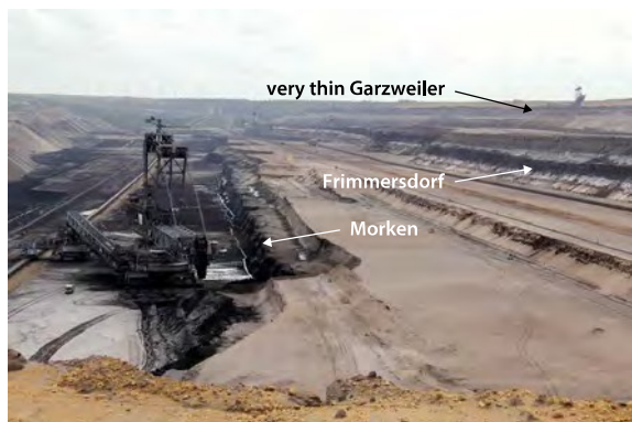
Figure 15.7. Picture of the opencast lignite mine of Garzweiler (Germany), exposing the Neogene sedimentary infill of the Lower Rhine Embayment and with the three regional lignite seams indicated. The location of the mine is given in Figure 15.6. Photo: Jan Stafleu.
