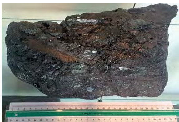
Figure 15.13. Picture of the last piece of produced coal, in custody of OneDyas, extracted from the Oranje-Nassau I mine on 31 December 1974, showing the centimetre-scale internal fracture (cleat) system of the coal. Production from this last operational mine in the Netherlands reached 427,000 tons coal in that last year. Photo: Richard Huis in 't Veld.
