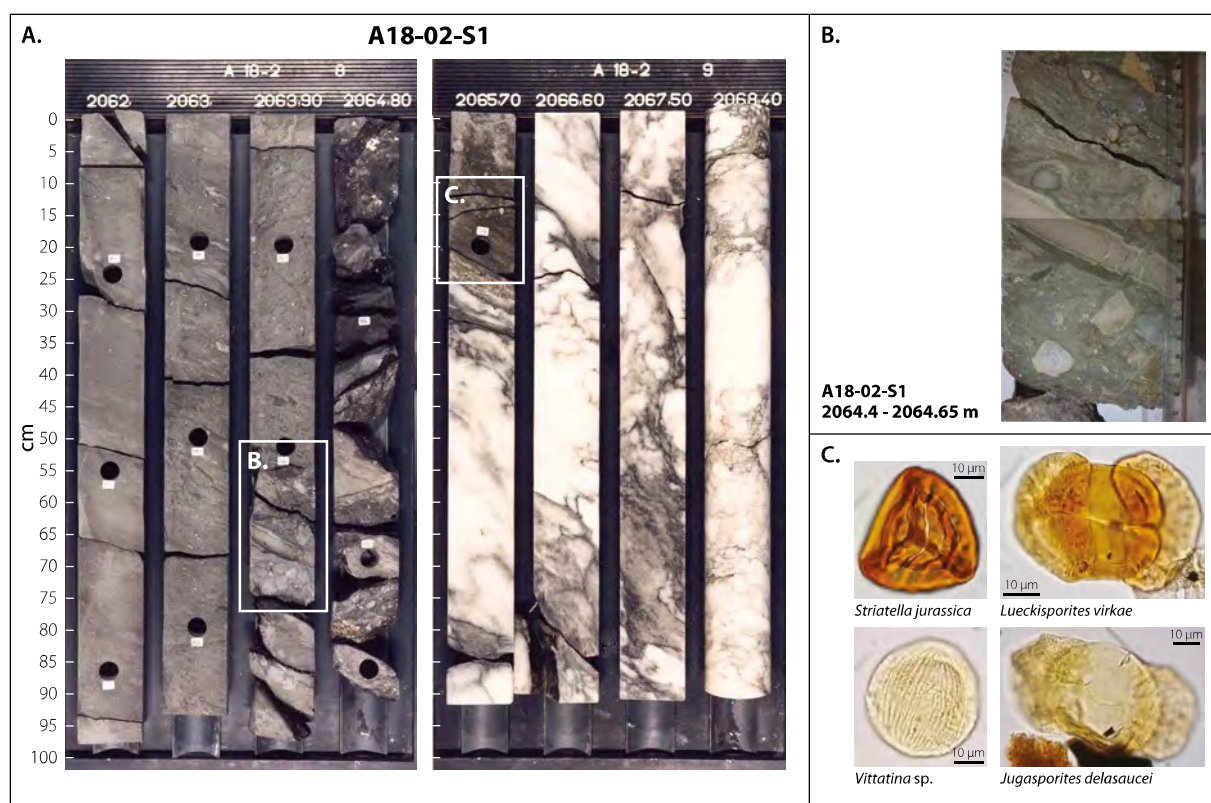
Figure 7.17. a) Core photographs of interval 2062.0-2069.3m of well A18-02-S1 from the Step Graben in the northern Dutch offshore (see Fig. 7.1 for location; source: nlog.nl). The core displays the unconformable contact between the Permian Zechstein Group (white) and the Upper Jurassic Scruff Group (grey and black). Core photos from www.nlog.nl. b) The base of the Upper Jurassic Schieland Group is represented by sandstones and breccias of the Noordsvaarder Member. Among the large and angular clasts are limestones and dolomites from the Zechstein Group. The sandy matrix contains dinoflagellate cysts that indicate a Volgian age. c) The base of the Upper Jurassic sequence is a dark, laminated claystone that contains excellently preserved pollen and spores from the Permian, e.g. Lueckisporites virkai , Vittatina sp. and Jugasporites delasaucei , in combination with Jurassic spores such as e.g. Striatella jurassica .
