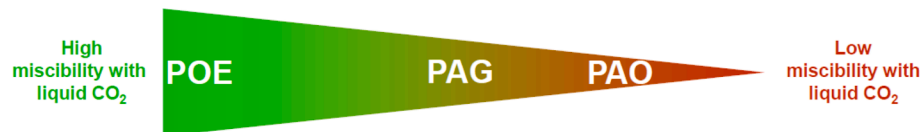
Fig. 25. Illustration of miscibility of CO 2 with different oils [159].
