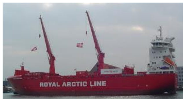
Figure 7 The small Feeder vessel "Mary Artica" with cargo handling cranes (588 TEU) [23].
