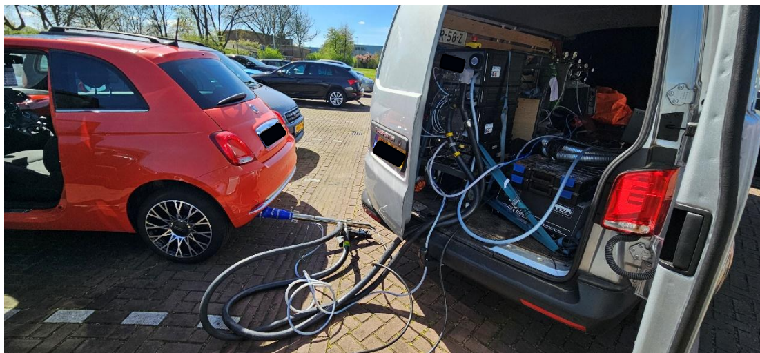
Figure 2.2: Image of the measurement equipment attached to a red Fiat 500 test vehicle. The flow tube and sampling lines of the PEMS and 5-gas analyser are directly connected to the red test vehicle, while the measurement equipment is located inside the rear cabin of the grey van. With this approach, the measurement equipment could quickly and easily be positioned next to a test vehicle.
