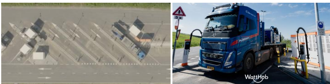
Figure 4.8: Truck parking and truck charging in the drive-through area (Picture source WattHub).
