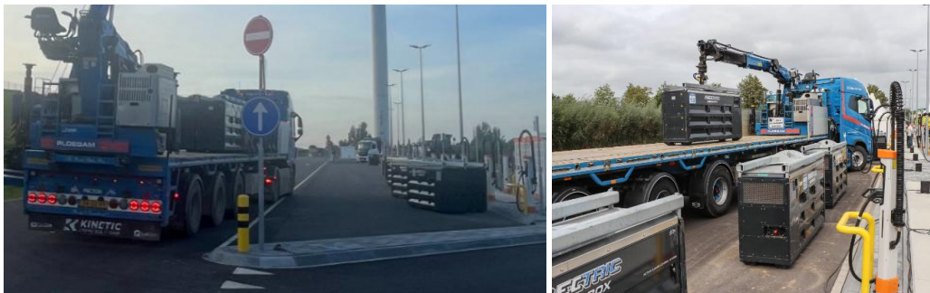
Figure 4.7: Truck exchanging the empty batteries for full at the battery charging area of WattHub (Picture source WattHub).
