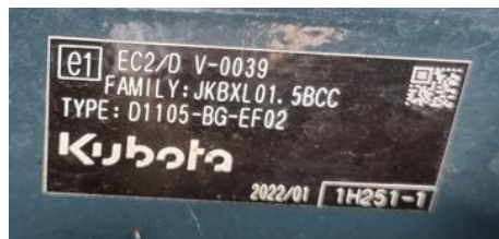
Figure 3.5: Engine plate of the Stage V Kubota diesel engine of the light pole.
