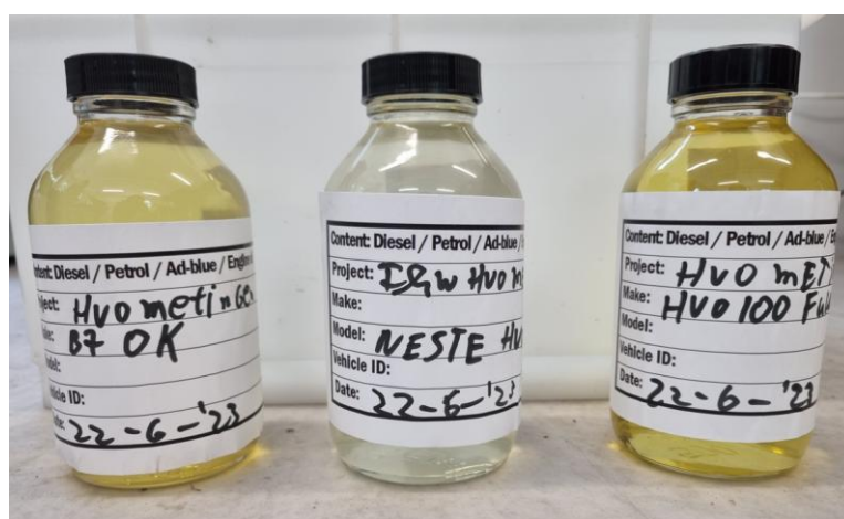
Figure 3.1: Samples of the three test fuels, from left to right: regular, fossil diesel B7 from OK, a 100% HVO from Neste (HVO1) and a 100% HVO from Full tank (HVO2).
