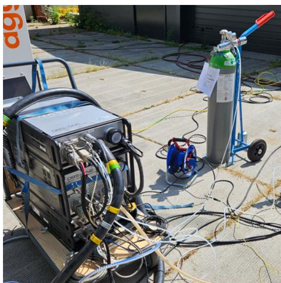
Figure 3.7: PEMS (Portable Emissions Measurement System), a Horiba OBS-one GS11.
