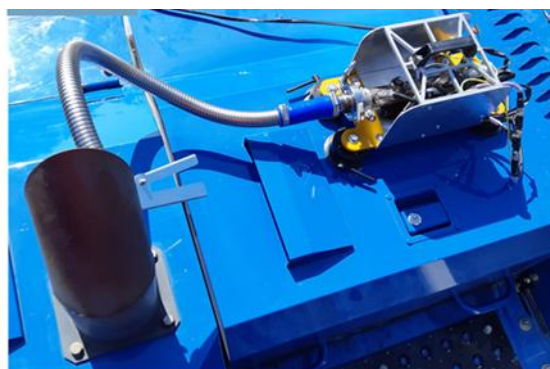
Figure 2.1: TNO's BOEMkit installed on a machine.
