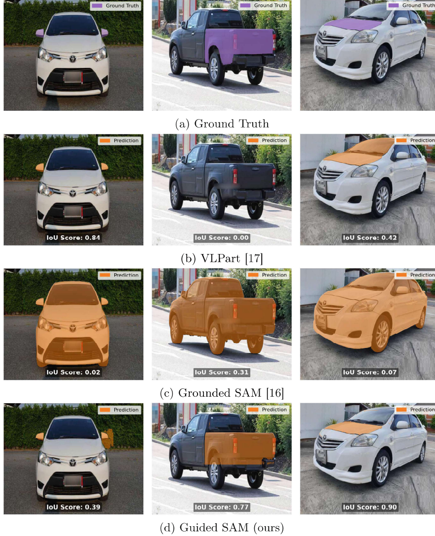
Fig. 5. VLPART either segments the object part very well or misses it completely, whereas Grounded SAM typically over-segments severely and often segments the full object. Guided SAM provides a balance, often segmenting the part well, while sometimes over-segmenting.
