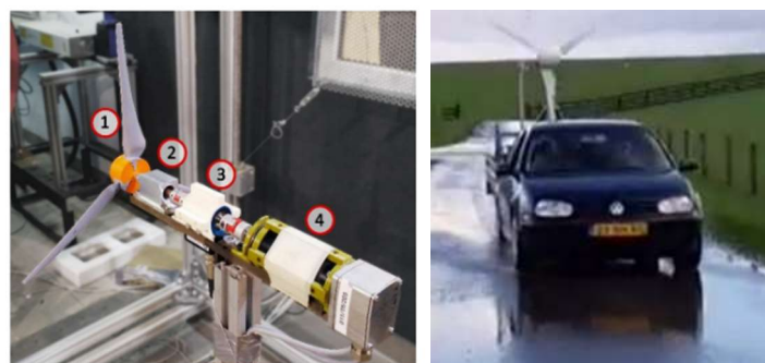
Figure 2: Left: wind tunnel test stand for preparatory analysis at Lodz University of Technology (1, 3D-printed rotor model; 2, bearing unit; 3, torque meter; 4, motor/generator) [4]. Right: Full scale testing rig of the NHL UAS on a trailer.
