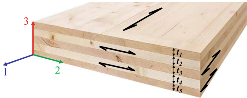
Fig. 1 Lay-up of CLT with the global coordinate system (1, 2, 3), layer numbers, and thicknesses. (Based on an image from [18])
