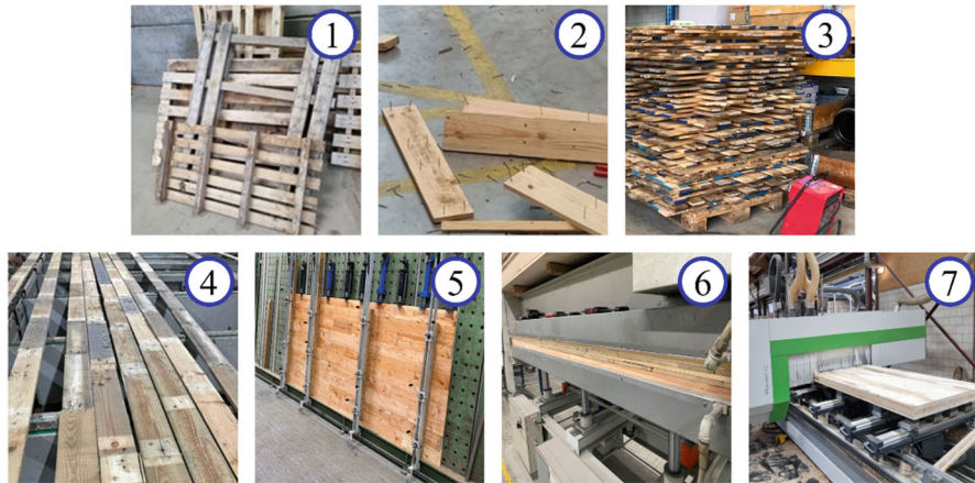
Fig. 2 Production process of C-CLT: (1) pallet acquisition, (2) disassembly and de-nailing, (3) drying, (4) finger-jointing, (5) edge-gluing, (6) face-gluing, and (7) planning and shaping
