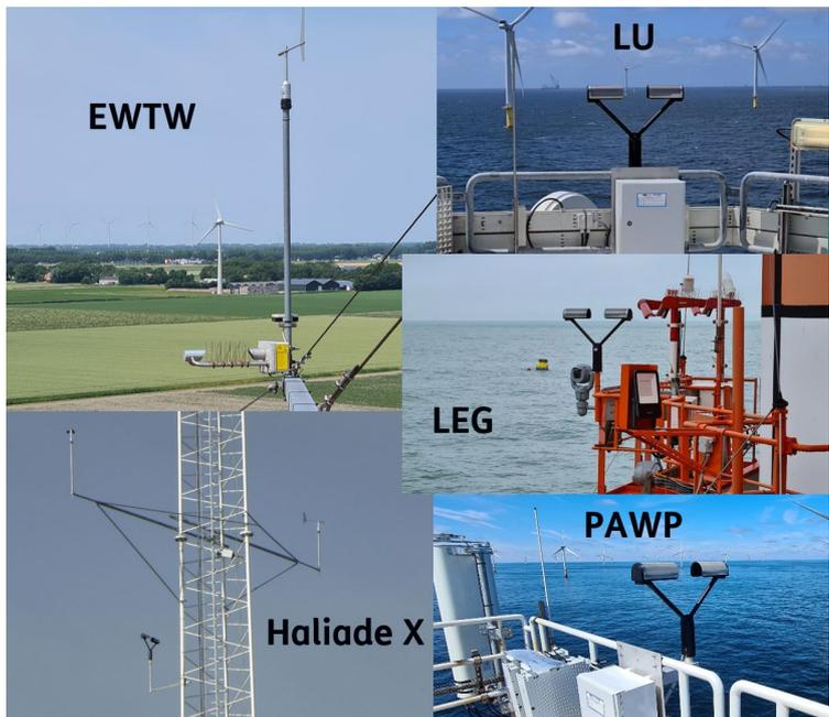
Figure 2 PROWESS precipitation network installed sensors.
