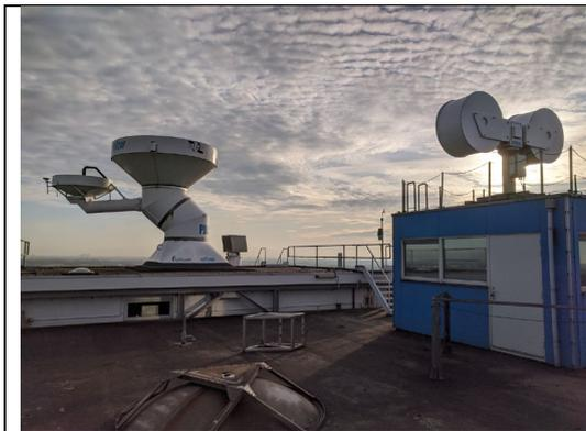
Figure 5- MESEWI radar (the one on the right of the image) installed on top of the EWI building at TU Delft
