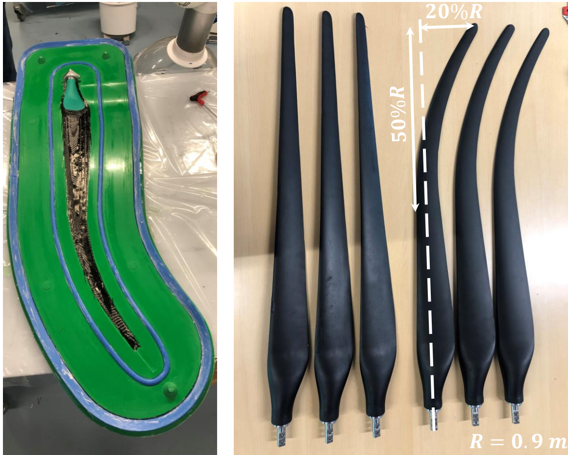
Carbon fibre-reinforced blades (vacuum-infused)
