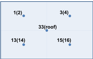
Figure C.3: Positions of pressure coefficients c_p for panel 11. The values in brackets represent the number of the channels on the down side of the panel. The position on the roof is located under the centre point of the panel.
