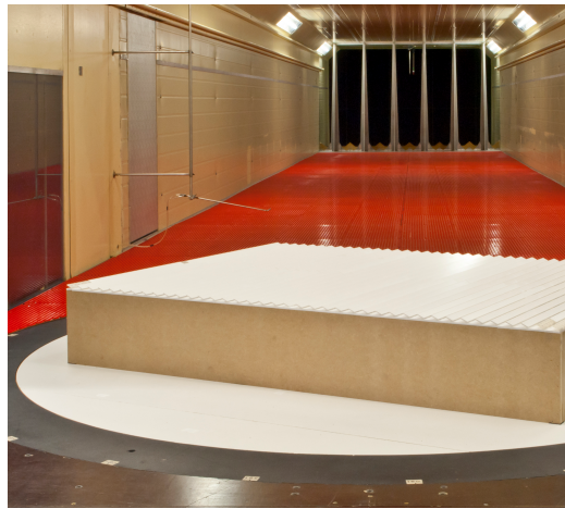
Figure 2.2: Photograph of a model with the roof covered with solar panels in the TNO wind tunnel in Apeldoorn.
