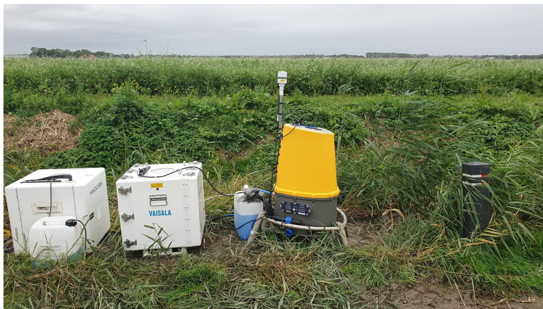
Figure 2.6: ZX 300M ZX1524 (right lidar in yellow) at the RSD verification location.
