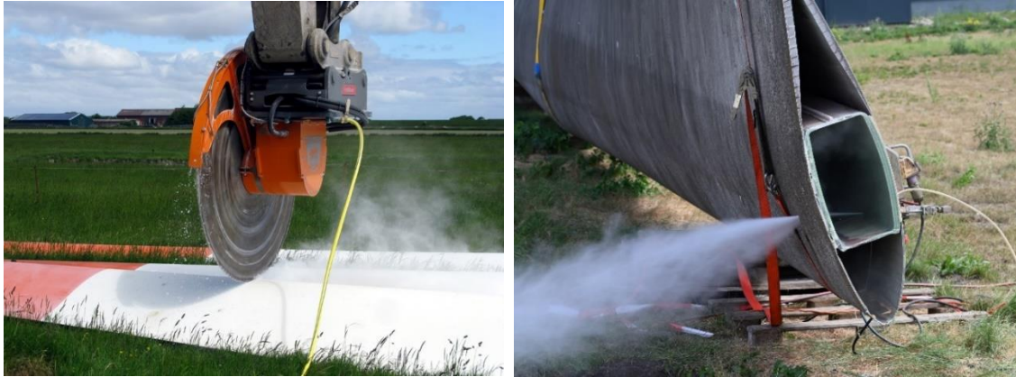
Figure 2.15: (Left) cutting a WTB with a rotating cutter disk (source Echidna); (right) water jet cutting of a WTB (TNO).
