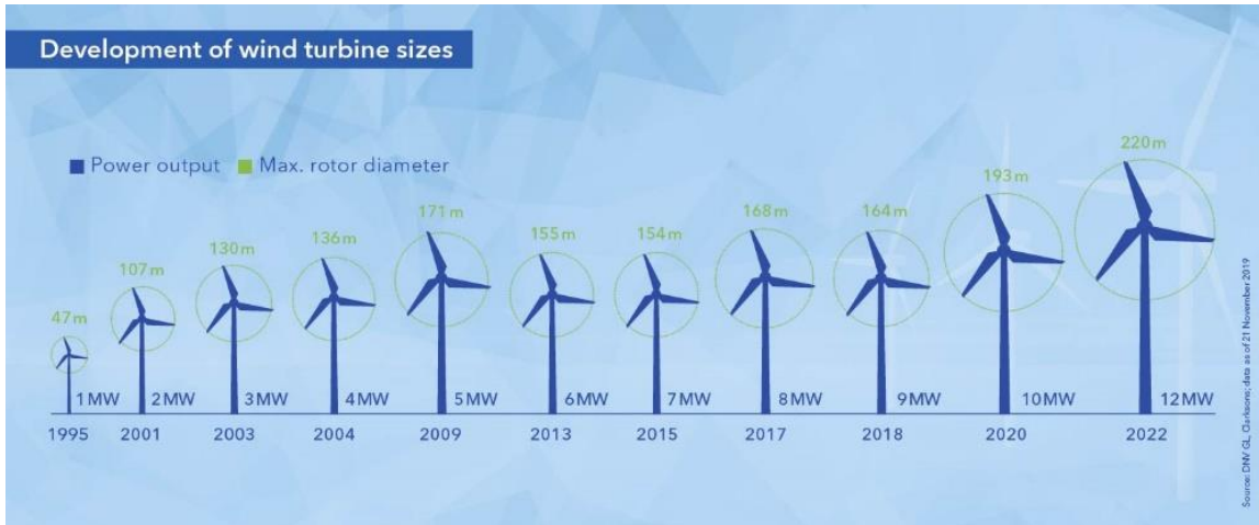
Figure 2.1: Evolution of the wind turbine rotor size from 1995 until now (source DNV).
