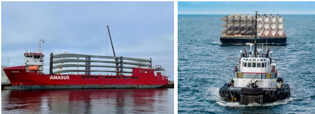
Figure 2.12: (Left) transport vessel with turbine blades (source Vattenfall); (right) transport on a barge with tug vessel (source North American Windpower).
