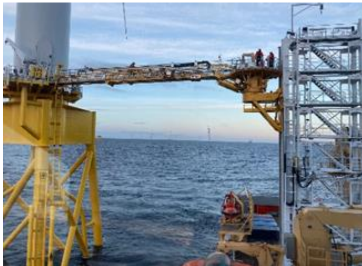
Figure 1.10: SMST L series gangway with height adjustment (courtesy of SMST)
