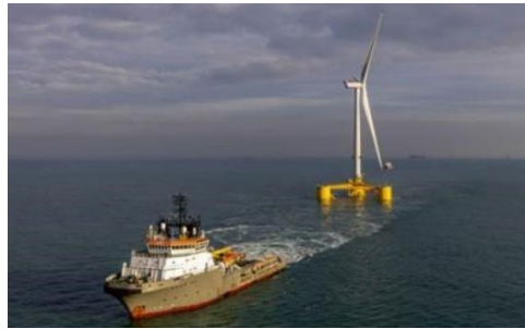
Figure 3.3: Towing operation at the Kincardine wind farm by Boskalis
