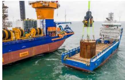
Figure 3.7: Active heave compensation by Sequalize for heavy lifting operations
