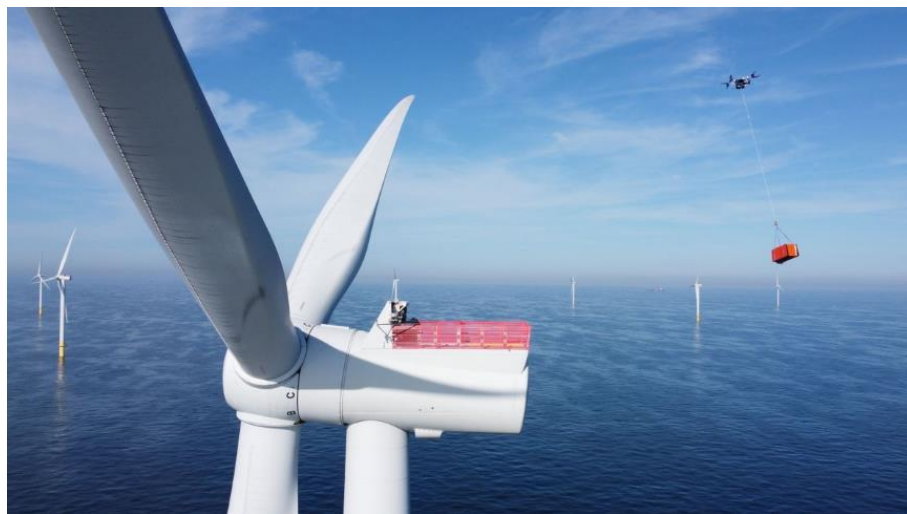
Figure 4.4: Heavy-lift drone transporting cargo from a vessel to the nacelle of a wind turbine [44]
