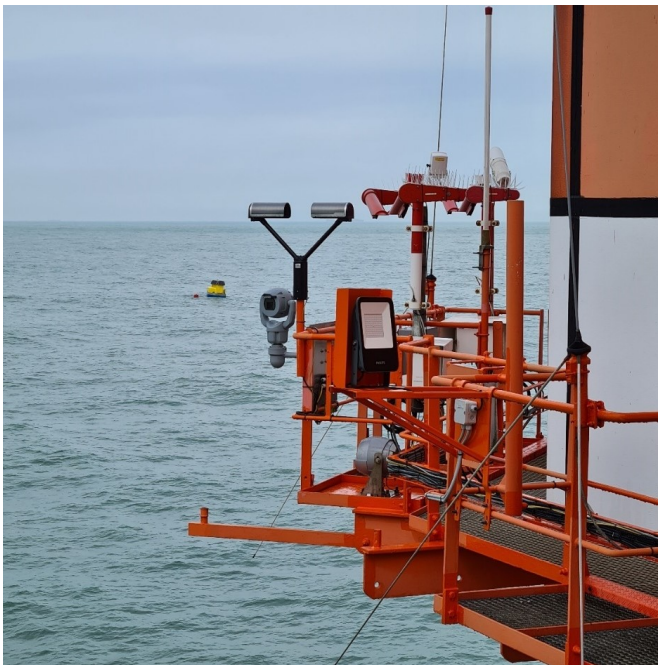
Figure 1.2: Disdrometer instrument installed at LEG platform.
