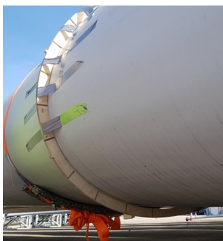
(a) Wooden template for drilling of holes for the pressure measurements
