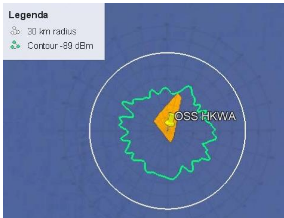
Figure 5.37 Coverage based on handheld situated at 2.5 m a.s.l.. Base station antenna height is 56 m a.s.l..
