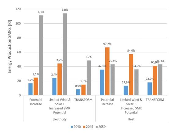
**Figure 3.5:** Electricity and heat supply from SMRs for the years 2040, 2045 and 2050 for the what-if analyses and TRANFORM. Above the bars the share is given of SMR electricity and heat supply in total national power and industrial heat (200-400 °C steam) production.
