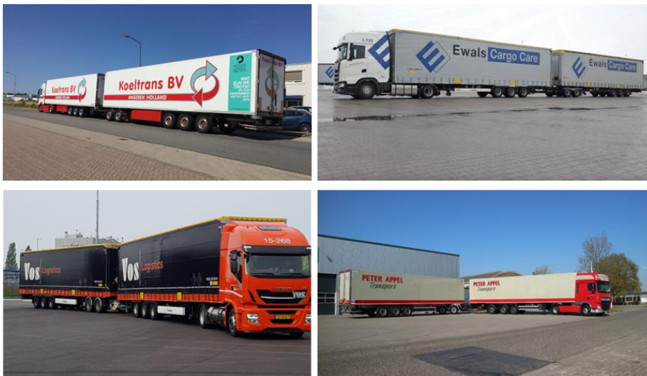
Figure 1.1: Illustrative examples of Dutch Super EcoCombi's (Van den Bongard & Janssen, 2019)
