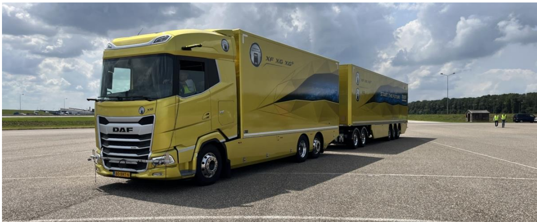
Figure 3.3: EcoCombi equipped with aerodynamic cabin 5
