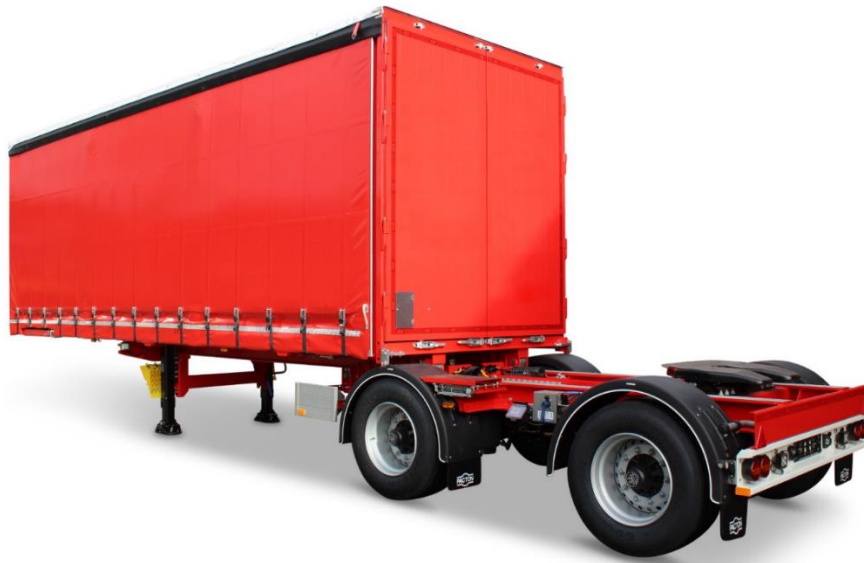
Figure 3.2: Link-trailer for B-double combination 4
