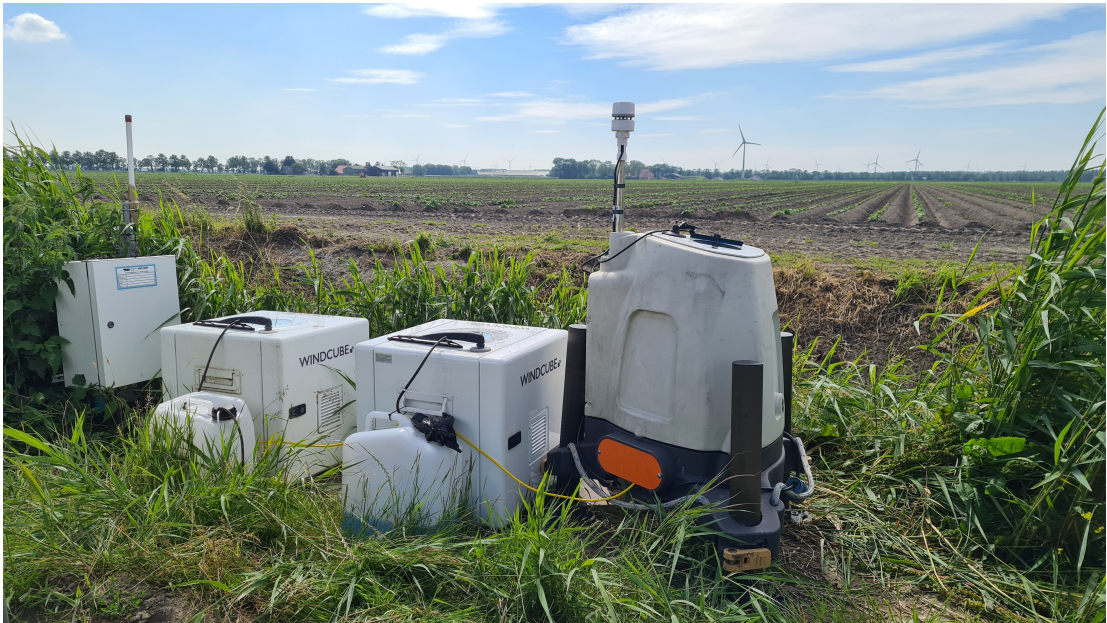
Figure 2.6: ZX 300 ZX315 (the lidar on the right) at the RSD verification location
