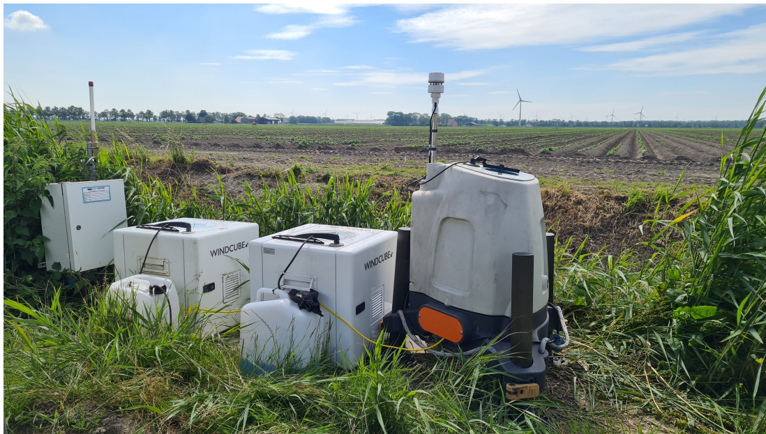
Figure 2.6: WindCube v2 WLS7-127 (the middle one) at the RSD verification location
