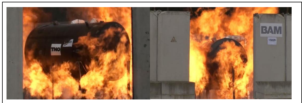
Figure 3 Screenshots, taken from the video registration, showing the double walled test tank fully engulfed in fire.
