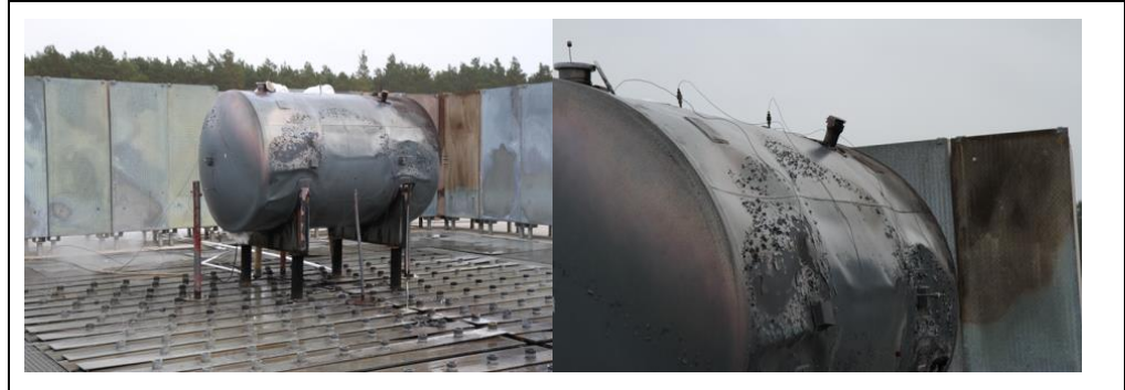
Figure 4 Images of the vacuum insulated double walled test tank.
