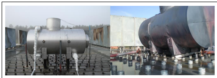
Figure 6 Impression of the single walled, Rockwool insulated test tank, before and after the experiment.
