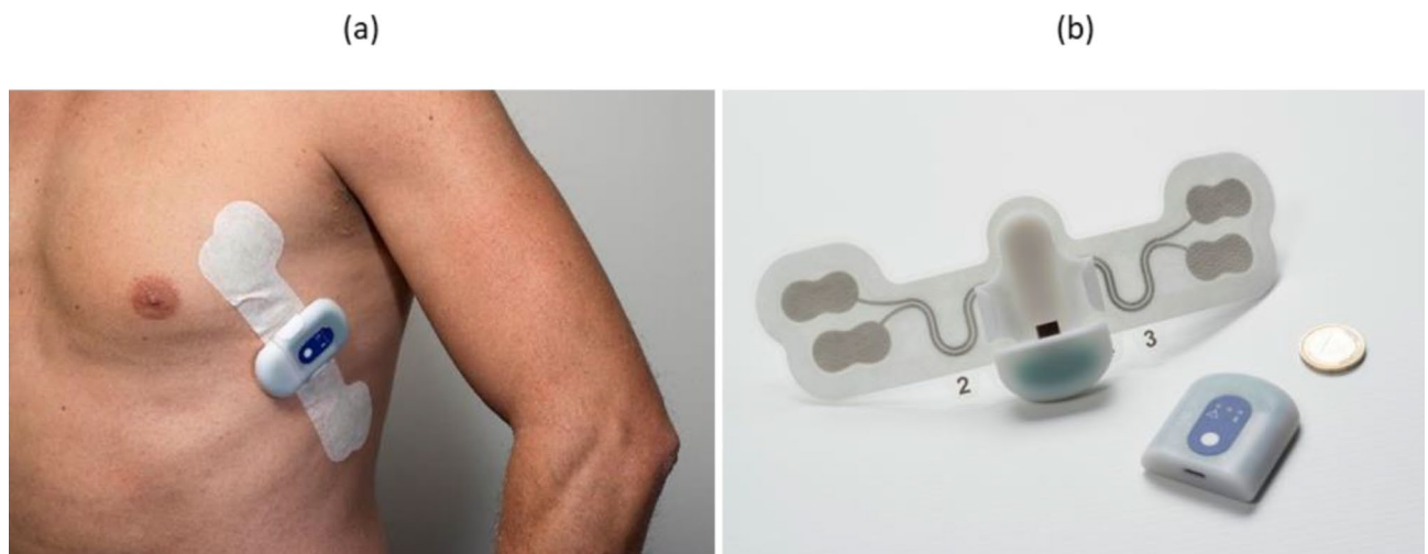
Fig. 8. (a) The Health Patch research platform adhered to the left side of the chest on a participant. (b) The Health Patch components such as a disposable part and re-usable part positioned alongside a coin to illustrate their size relative to a scale).
