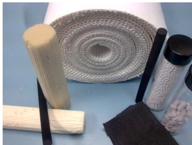
Fig. 2. Illustration of a variety of adsorbent structures including (left to right): ceramic and carbon adsorbent monoliths, corrugated paper monoliths (center), fabric adsorbent and conventional beaded adsorbents. Reprinted with permission from Rezaei and Webley (2010) [12].
