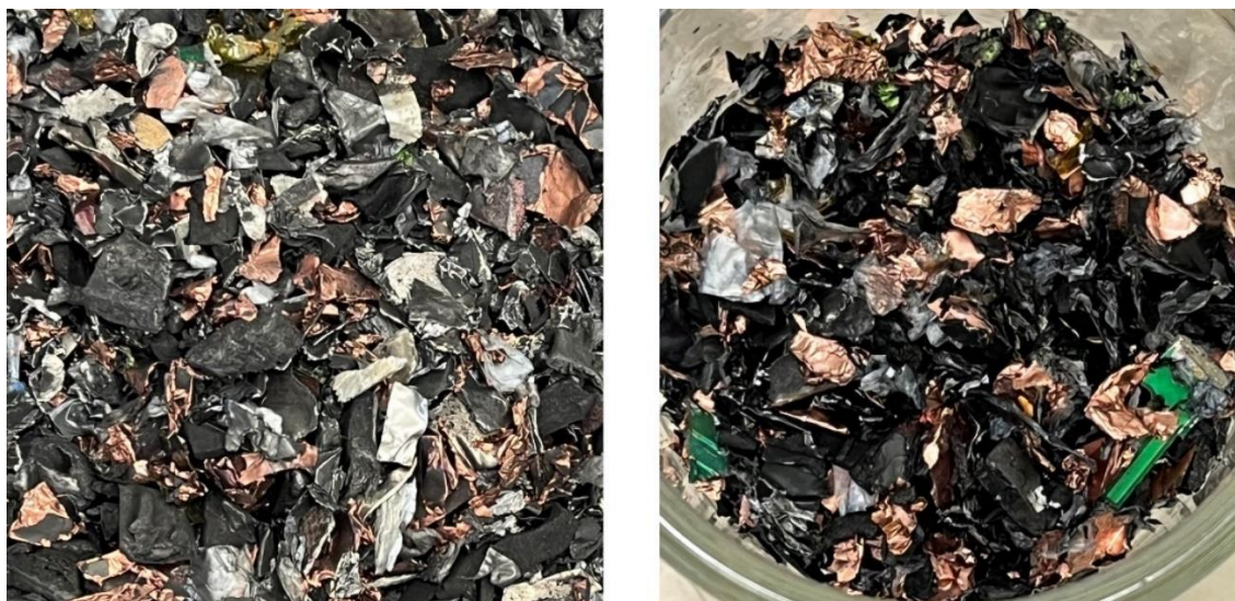
Figure 19: The appearance of coarse fraction material before (left) and after (right) recovery process.
