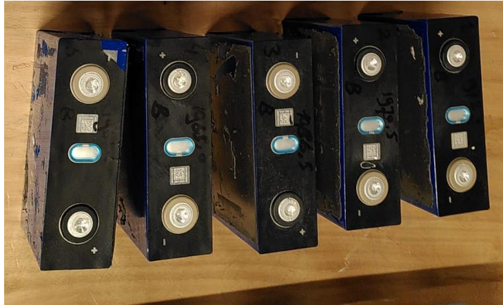
Figure 7: The prismatic LFP battery cells that were used for trials 5 and 6.
