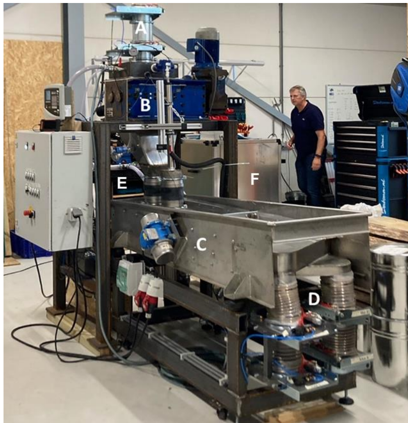
Figure 1: Image of the battery pretreatment setup with the battery inlet (A), battery shredder (B), sieving table (C) and solid fraction collection (D), condenser (E, on the back of the setup), and activated carbon filters (F) indicated.
