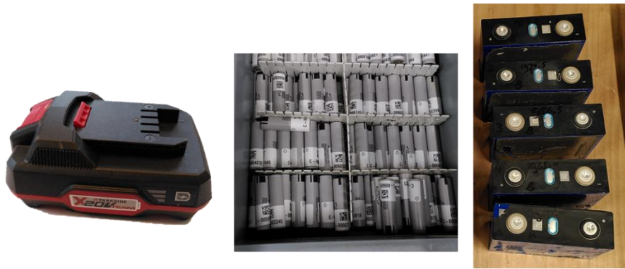
Figure 2: Different battery types that were used for the different trials with NMC batteries in casing (left), cylindric NCA cells (middle), and large prismatic LFP cells (right).
