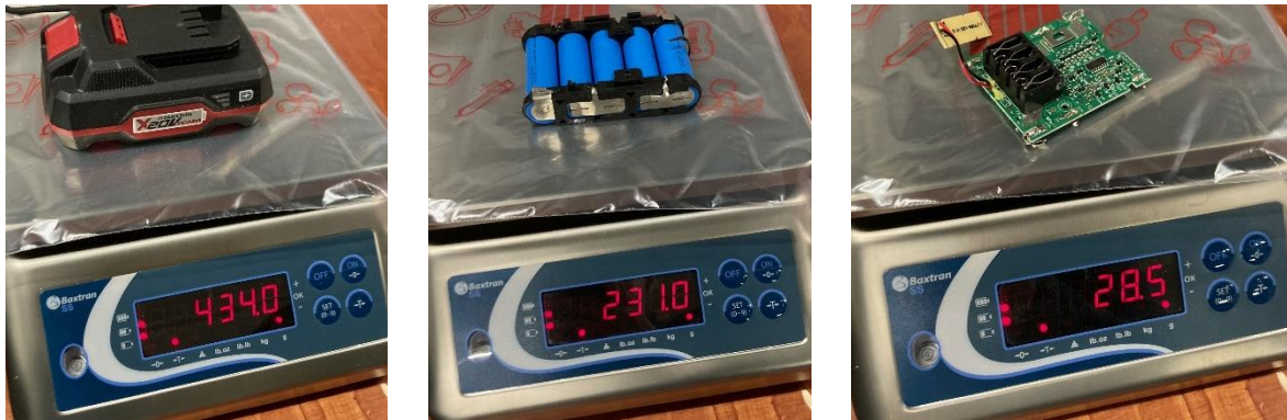
Figure 5: The mass of the NMC battery packs (left), the individual NMC battery cells within one pack (middle), and the mass of the battery management system within one battery pack (right).
