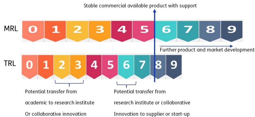
Figure 3 – Potential tech transfer/hand-over in innovation projects leading to commercial available products or services
