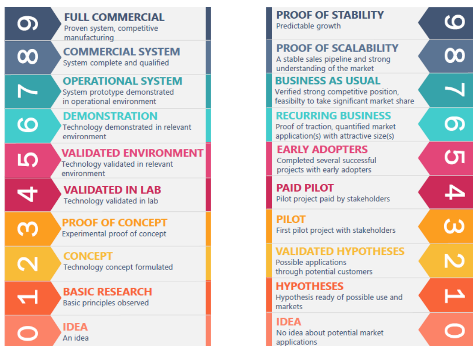
Figure 1 – On the left side the TRL scale & on the right side the MRL scale (source: TNO tech-transfer 3 )
