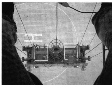
Figure 4.2 Crane driver's view on hoist and spreaders
