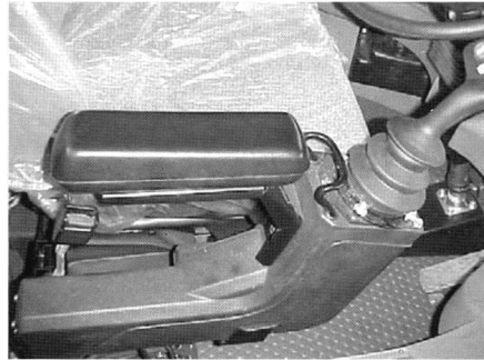
Figure 6.8 A console mounted armrest has poor adjustment qualities (here mounted in a wheelloader)
