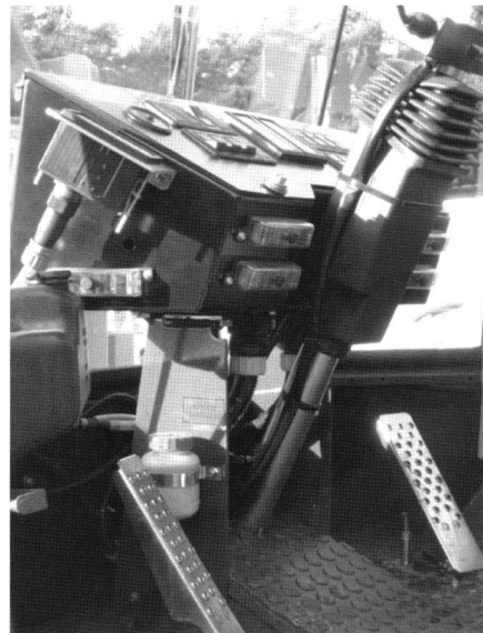
Figure 6.4 The new adjustable steering column
