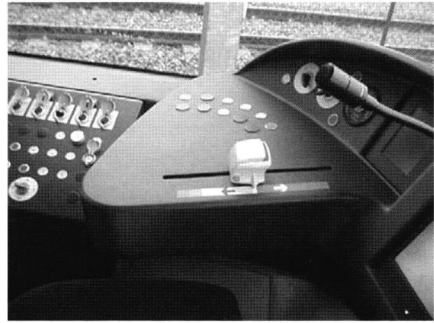
Figure 3.4 Emergency-stop, integrated in the drive-stop handle
