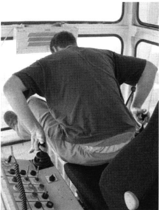
Figure 4.5 Crane driver operating the crane in extreme posture
