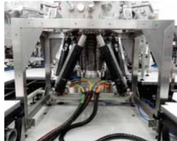
Figure 7 Hexapod and bellow installed underneath the exposure chamber.
