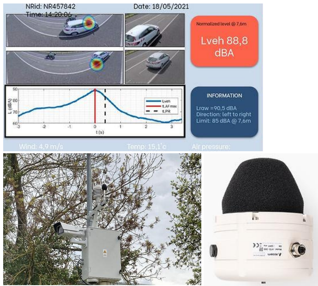
Figuur 3.3: Acoem Noise camera (Bron: website Acoustic1.co.uk).
