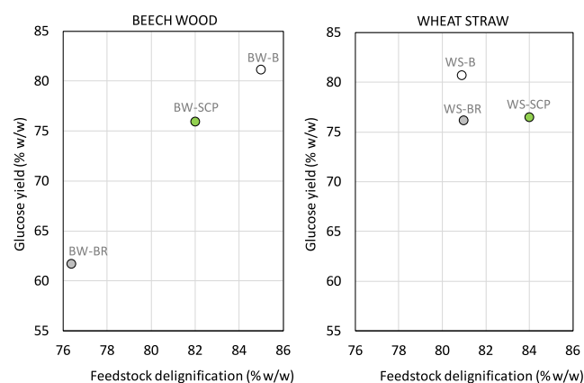
Figure 8. Enzymatic saccharification of pulps; correlation glucose yield and feedstock delignification of BW and WS pulps.
