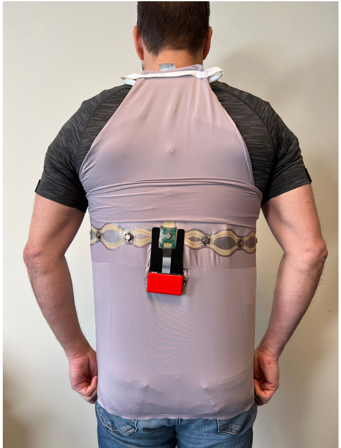
Fig 1. The MYSA system. Location of the six vibration motors across the middle of the back and the control box (red) containing the printed circuit board and battery.
