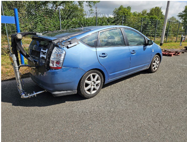
Figure 3.1: The Toyota Prius test vehicle equipped with PEMS test equipment ready for on-road testing
