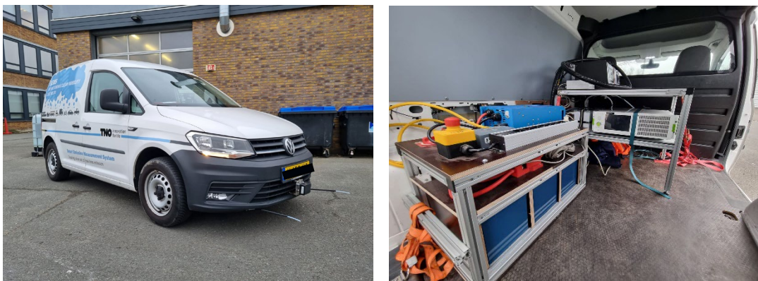
Figure 2.1: The inlets and radar on the front bumper and the license plate camera behind the window (left), and the measurement equipment and battery pack in the rear cabin (right) of the TNO plume chase vehicle.
